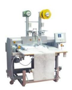
A major advantage of this new process is to be able to lay the rovings according to the distribution of forces within a structural component. [67.]
