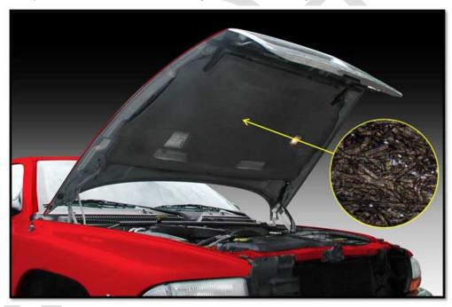
controls the mid and high frequency wavelength by managing the sound pressure level variations and 'trapping' the energy in the insulation layer of the part. This makes the composite more efficient than just the Homogeneous insulation material by itself.
